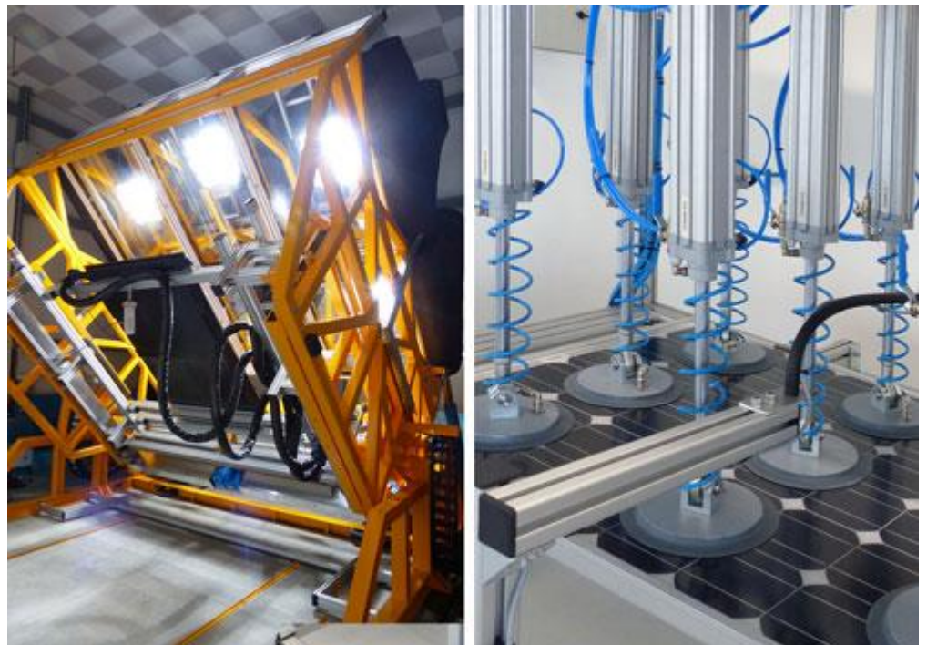
PSEs steady state solar simulator SORAS-ST6 and mechanical load tester MLT12 are part of the test center of Grupo ICE in Costa Rica. © PSE AG
